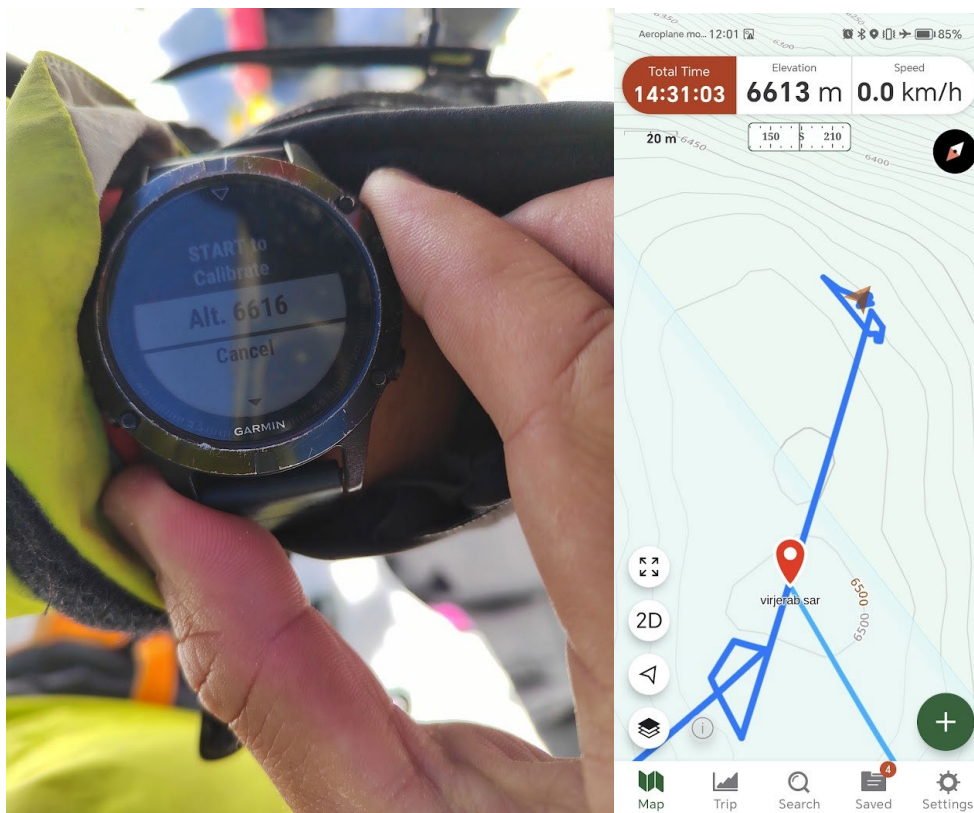
Garmin Calibrated off GPS at 6616m and the phone shows 6613m,
