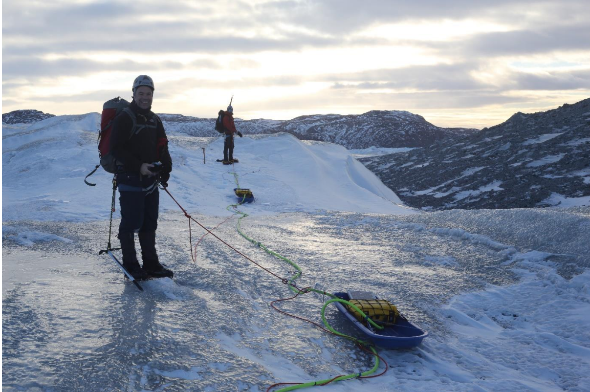
Figure 3. Ice Radar system set up. The radar transmitter and receiver are each housed in a plastic pulk, separated by approximately 20 m. The radar antennas are attached to climbing cord which connects the pulks and radar transmitter and receiver, and also extends in front of and behind them. The whole system is loosely attached to a 60 m climbing rope to which expedition members are attached. (Photo: Andrew Sole)
